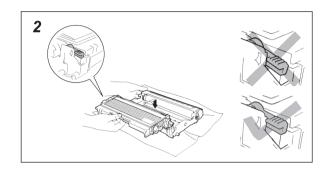
2. Unpack a new drum unit. Install the cartridge into the drum unit properly as shown in the figure above.
