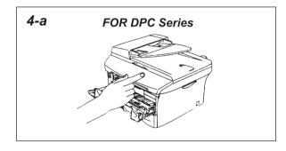
4-a. Reset the drum counter: Keep the machine on and press Options on the control panel. When the LCD shows "Replace Drum?", press ②. Close the front cover after "Accepted" shows.
