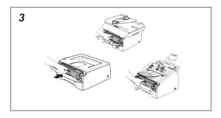
3. Install the drum unit and toner cartridge assembly into the machine. DO NOT close the machine front cover.
