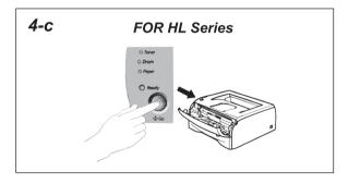
4-c. Reset the drum counter: Keep the machine on and press the Go button for at least 4 seconds until all the LEDs are on. Close the front cover after the Drum LED is off.
