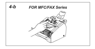
4-b. Reset the drum counter: Keep the machine on and press Options on the control panel. When the LCD shows "Replace Drum?", press 1. Close the front cover after "Accepted" shows.
