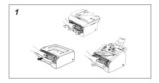
1. Remove the drum unit and toner cartridge assembly from the printer and separate the cartridge from the drum unit according to instructions in the machine manual.
