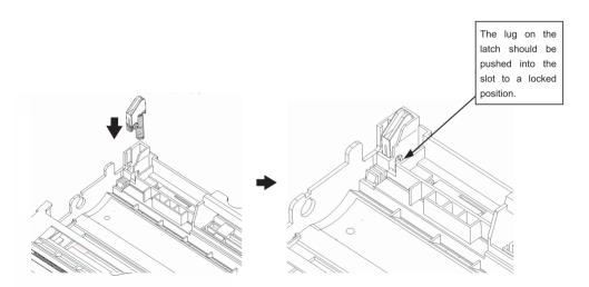
2. Put the 2 latches (with spring fixed) into the slot on each side of the drum unit as indicated.
